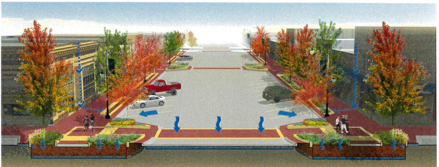
Streetscape master plan graphic showing stormwater management strategies for a reconfigured downtown in Mapleton, Iowa.
